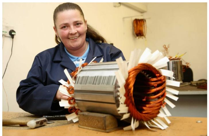
Each winding is then subjected to 2000V-to-earth flash test, ohms readings are taken with a multi-meter and recorded, and then the winding is subjected to a full load test on a transformer.
