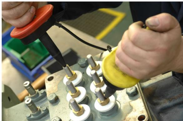
■ The compressor is then transferred to our Test Centre where it is subject to the most rigorous testing procedure on our unique, purpose-built test rig both open and under load. At this stage the compressor performance is recorded on the Rebuild & Test Certificate;
